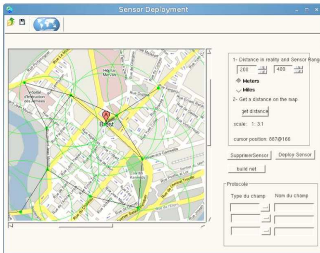
Figure 1. From distribution to connectivity: node distribution is decided to obtain wireless connections. Circles represent area where other sensors can (likely) receive the center messages.
